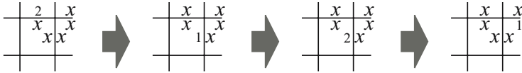
Fig. 7. An internal signal propagating in a TSE in state q_0 . Only part of the TSE loop is shown to save space.
